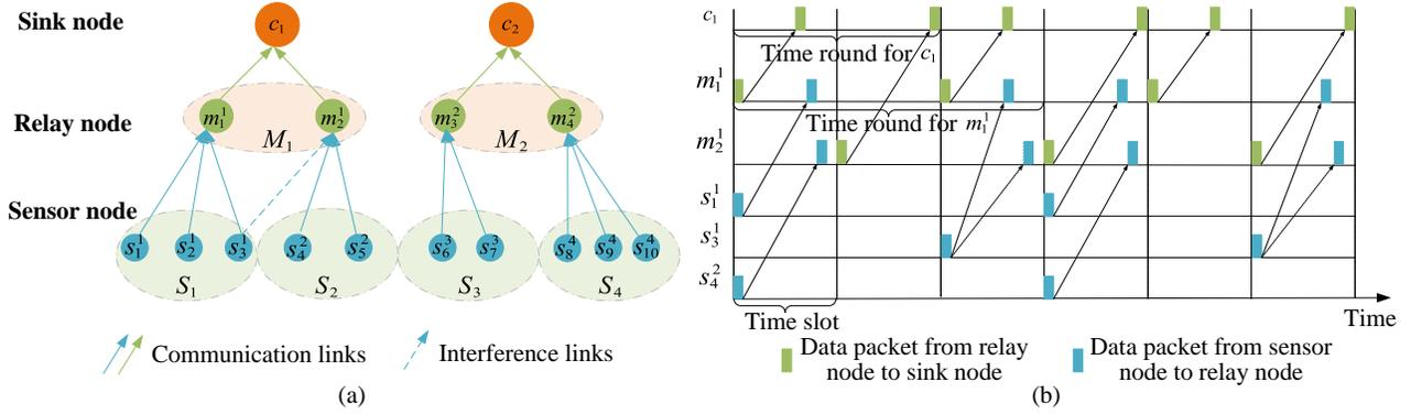
Fig. 2. An example of the static network topology and the TDMA protocol: a) The static network topology; b) The packet scheduling strategy in TDMA protocol.
