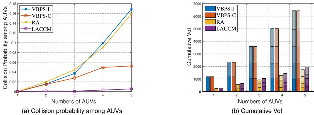
Fig. 6. Collision probability among AUVs and cumulative VoI performance with different numbers of AUVs.
